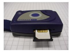
Place the SIM card into the holder and push the holder back into the device.
