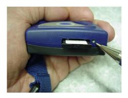
Press the switch indicated in the picture. The SIM card holder comes out.
