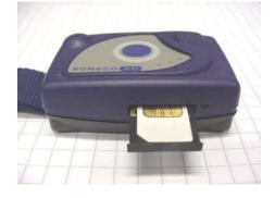
Insert a SIM to the holder and push the holder in to CC3 until it locks.
