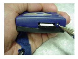
Push the yellow dot with a pin in order to eject the SIM card holder
