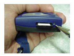
Push the yellow dot with a pin in order to eject the SIM card holder
