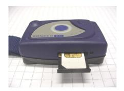
Insert a SIM to the holder and push the holder in to CC3 until it locks.
